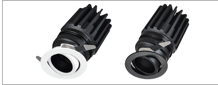
투링 55 LAMP 10W,15W,20W SIZE 63X H93/130 CUT SIZE 55 BEAM ANGLE 24°, 36°, 50°
