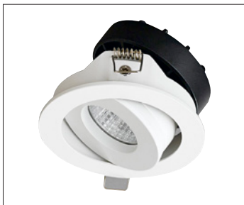
스통원형 95 LAMP 15W SIZE 105X65 CUT SIZE 95 BEAM ANGLE 24°
